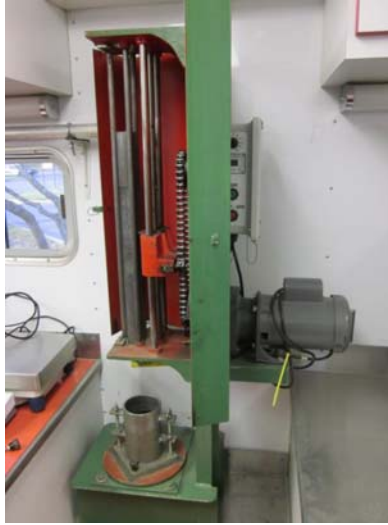
Figure 15. Mechanical Proctor setup
