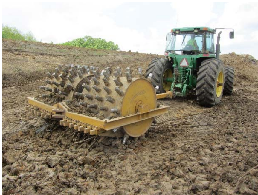
Figure 33. Sheepfoot roller used for soil compaction
