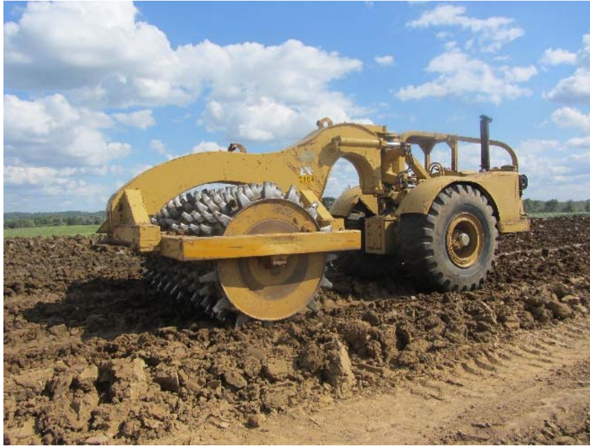
Figure 56. Sheepfoot roller used for soil compaction
