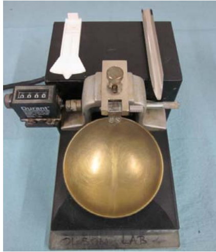
Figure 14. Atterberg limits test
