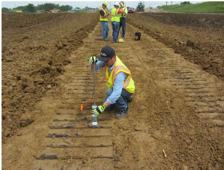
Figure 73. ISU in situ drive cylinder test
