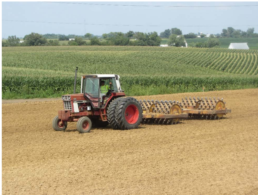
Figure 110. Sheepfoot roller used for soil compaction
