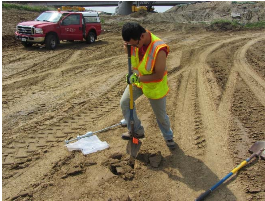
Figure 81. ISU in situ drive cylinder test
